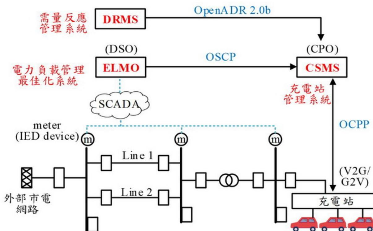
Figure 1. The schematic diagram of integrated structure for EV charging facilities.
