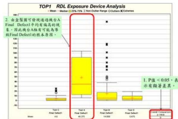
Fig.3 Top1 RDL exposure process device analysis
