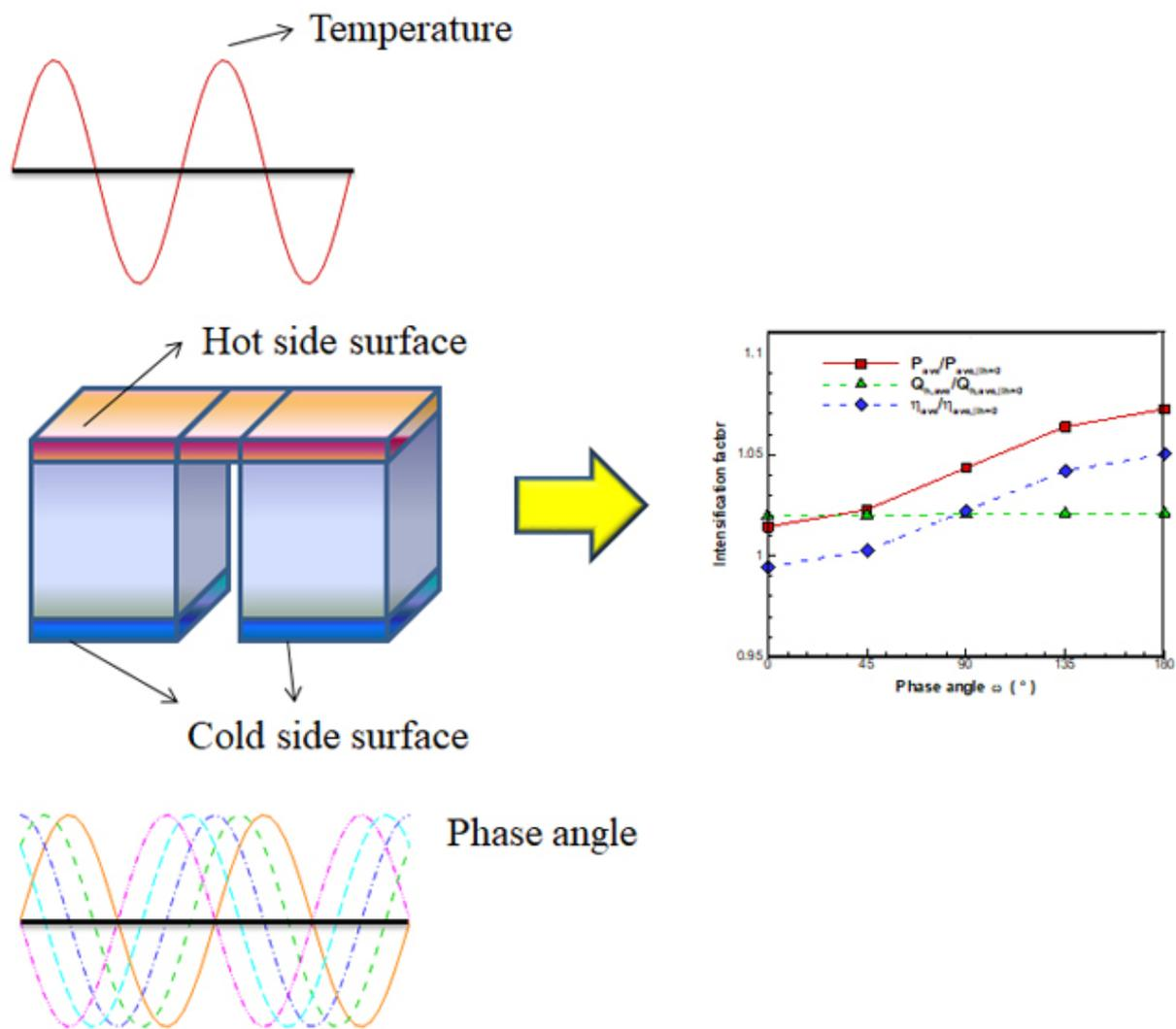
Figure 1. A schematic of temperature oscillation on the surfaces of a TEG and its performance.
