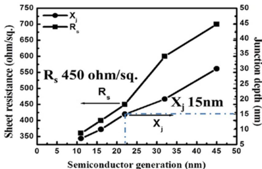
Figure 1 Current trends in semiconductors with regard to  $X_j$  and  $R_s$
