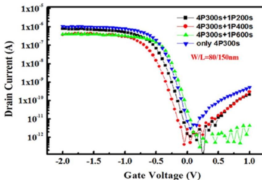
Figure 6 The IDVG curves of P-MOS devices produced with different MWA processes
