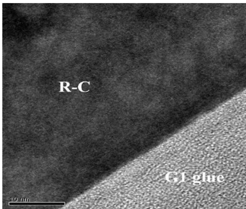
**Figure 2** The thickness of the amorphous layer in a TEM cross section image after 2400 W MWA for 300 s
