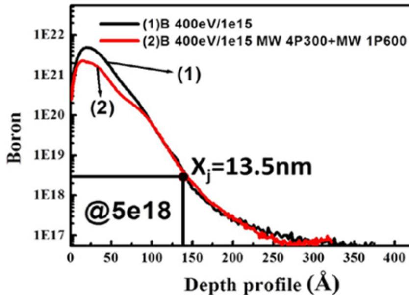
Figure 5 The SIMS profile of the implanted silicon before and after two-steps MWA
