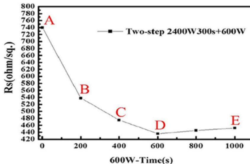
Figure 4 The sheet resistance of samples after two-steps annealing
