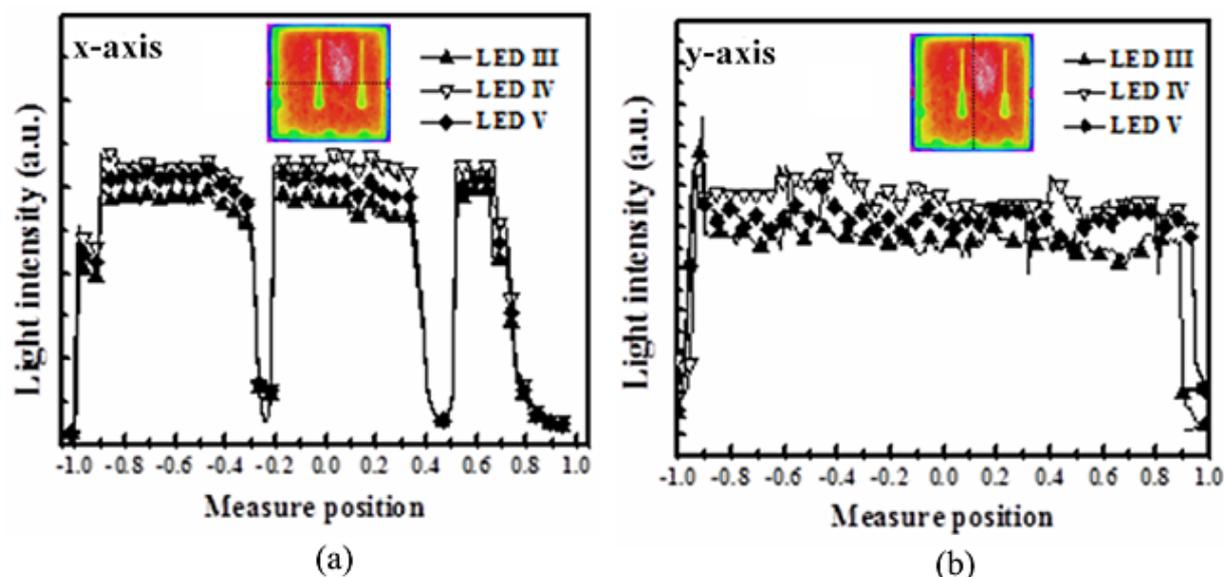
Fig. 2. Spatial profiles of light emission intensity taken from LED III, LED IV, and LED V under an injection current of 350 mA in the (a) x-direction and (b) y-direction.
