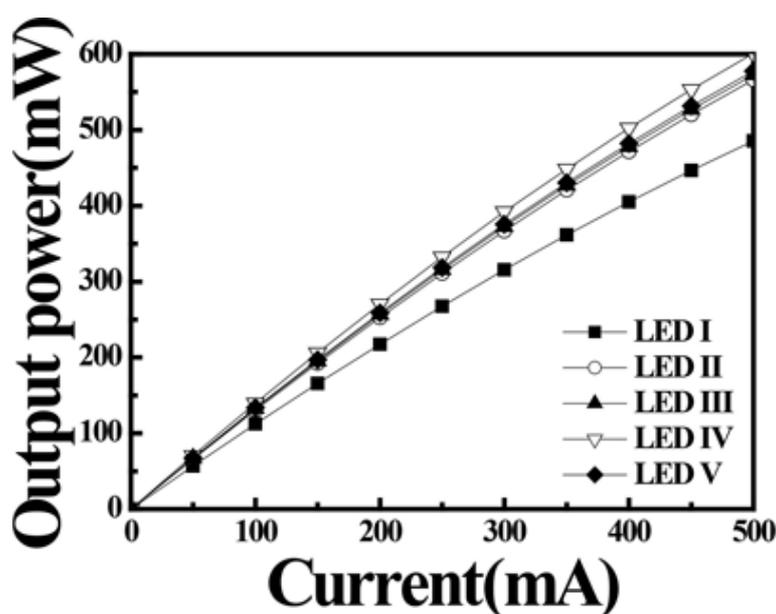
Fig. 1. Output power as a function of injection current for the five LEDs.
