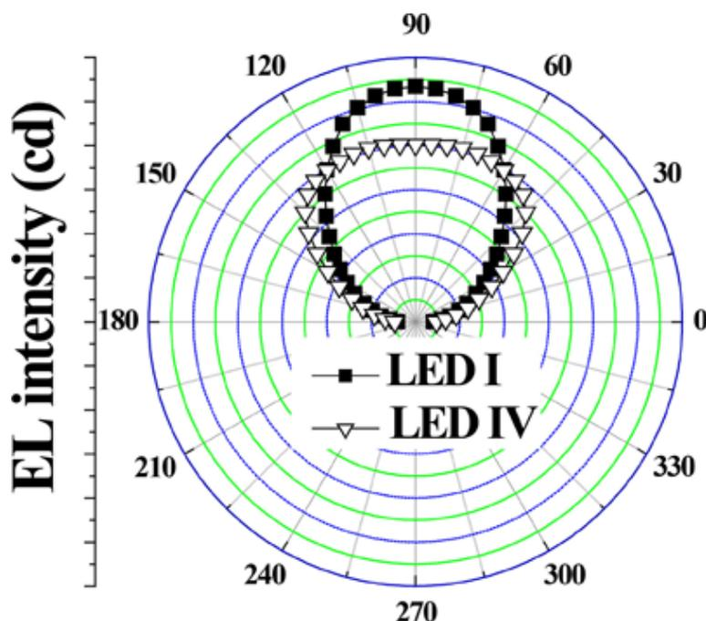
Fig. 3. Light output patterns measured from the two LEDs.
