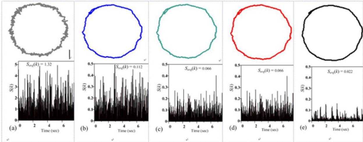
Fig. 2. Comparison of smooth trajectories and  $S(k)$  associated with circular motion determined by various methods. (a) Raw data. (b) MAF method. (c) KF method. (d) STKF method. (e) FLASTKF method.
