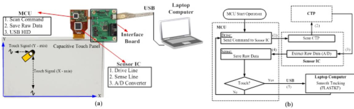
Fig. 1. (a) Photograph of the experimental CTP system. (b) Block diagram of the CTP system.
