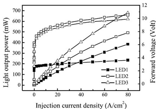
Fig. 2. L-I-V characteristics measured from the three fabricated LEDs.
