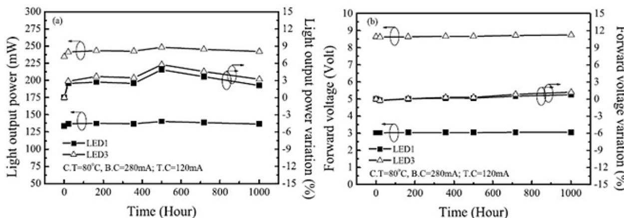
Fig. 3. Life-test results for (a) output power and (b) forward voltage for LED1 and LED3.
