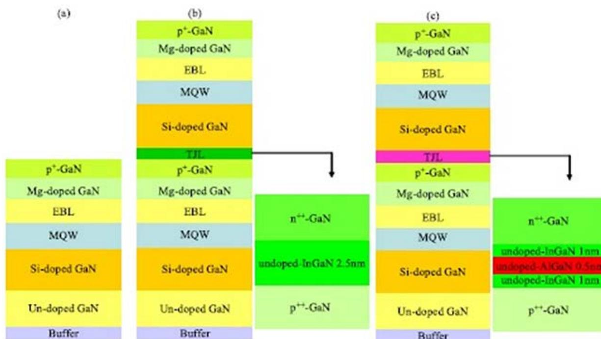
Fig. 1. Schematic diagrams of (a) LED 1, (b) LED 2, and (c) LED 3.
