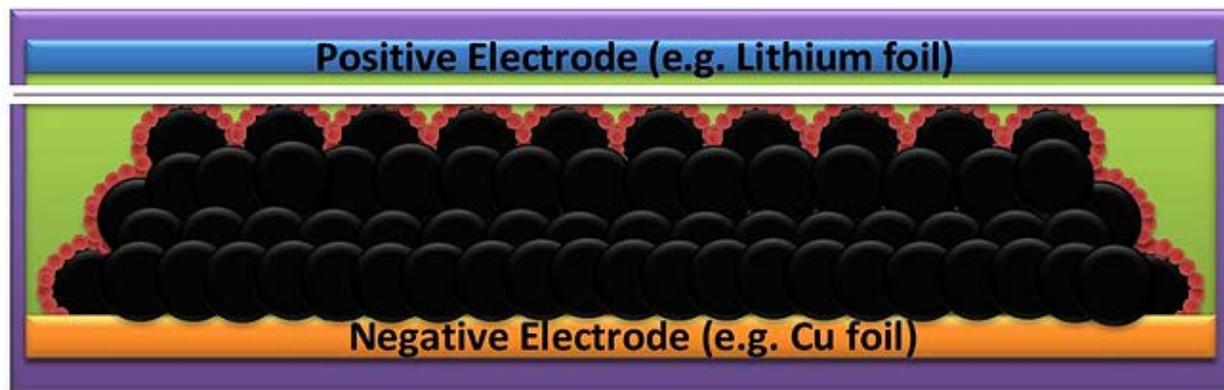
Figure 1. Schematic for a lithium ion battery with the anode coated with an electrically conductive nitrogen-incorporated ultrananocrystalline diamond film.
