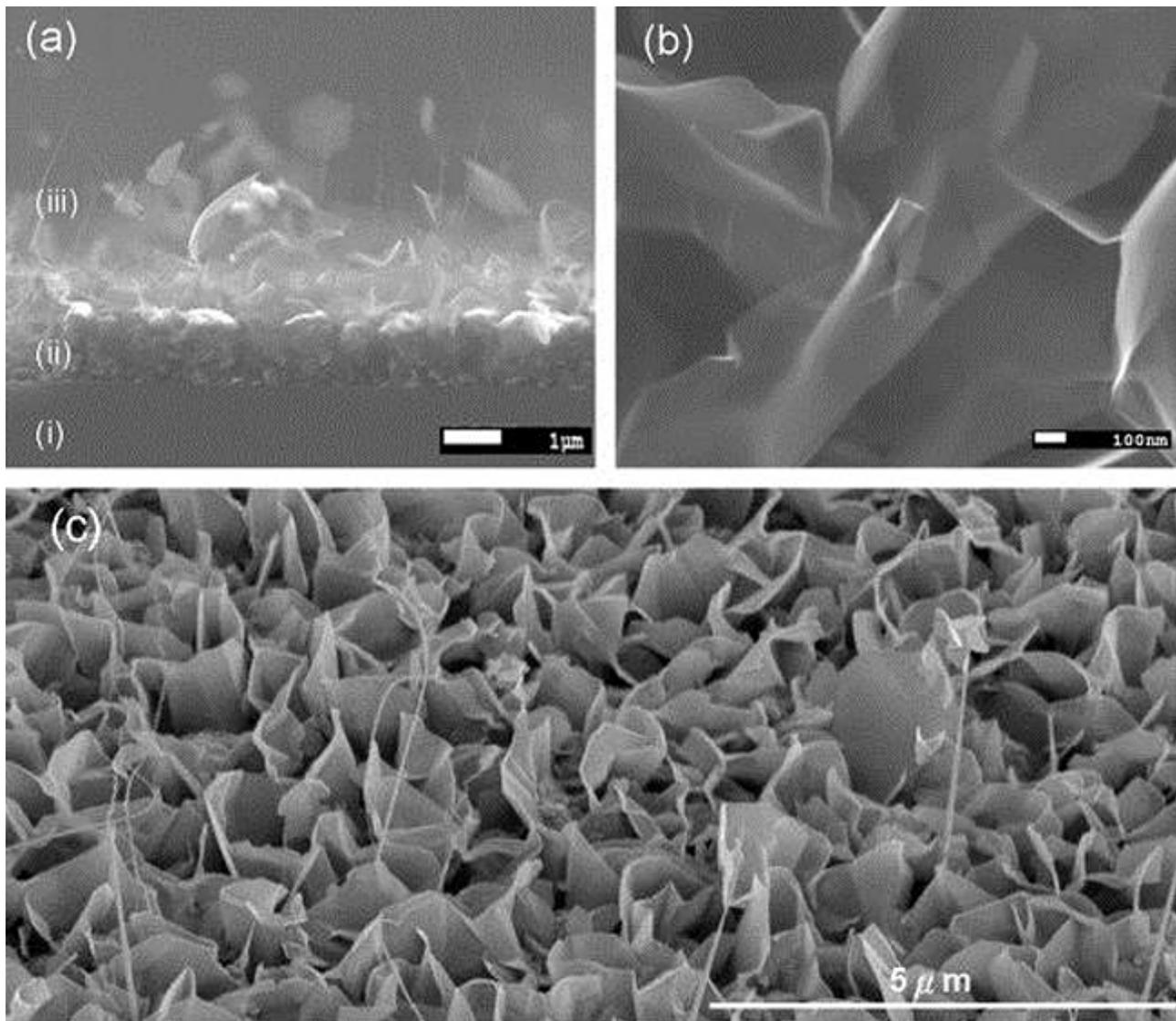
Figure 1. SEM image of standing graphene nanowalls grown on a CVD diamond film.
