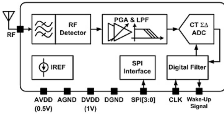
Block diagram of Wake-Up Receiver.
