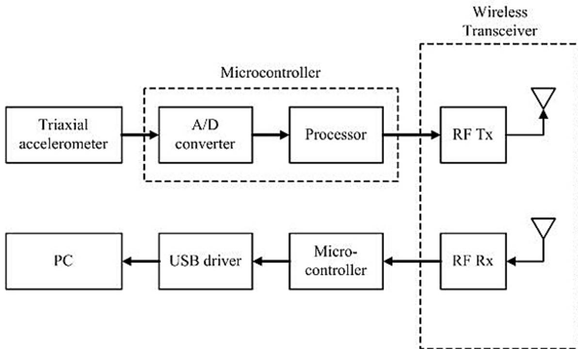
Fig. 2 The schematic diagram of the digital pen module.
