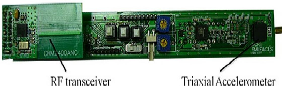
Fig. 1. The circuit board of the digital pen.
