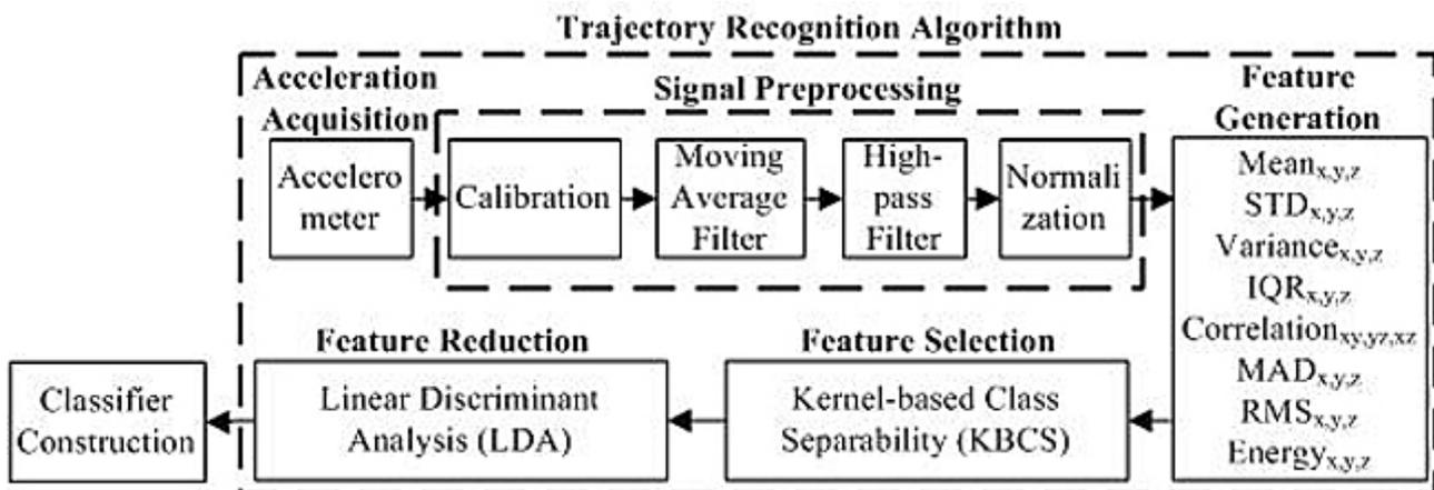
Fig. 3 Block diagram of the trajectory recognition algorithm.
