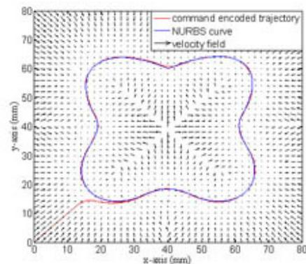
Fig. 4. Blue line: 4-leaf clover contour represented in NURBS form;  $h$ : 2 mm. Red line: trajectory encoded by velocity field; initial point (0,0)
