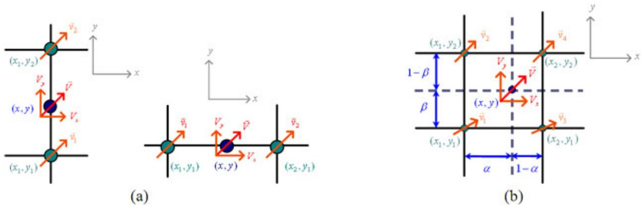
Fig. 2. Desired velocity field (a). point  $(x,y)$  located between two nearby grid points. (b). point  $(x,y)$  located inside a rectangle consisting of four grid points.
