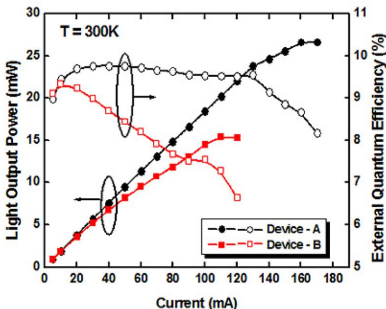
Figure 3 Light output power and external quantum efficiency as a function of DC injection current.
