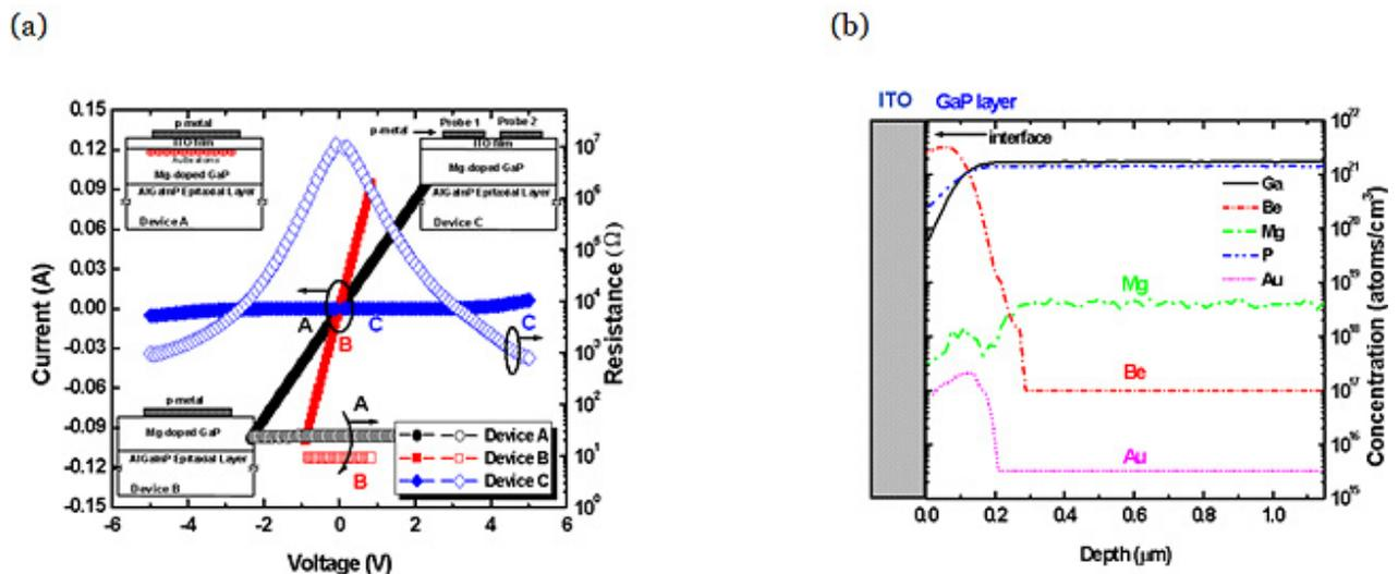
Figure 1 (a) I-V characteristics of contact resistances for the studied LEDs. The inset shows the simplified schematic diagrams for studied devices. (b) The depth profiles, by SIMS measurement, for device A.
