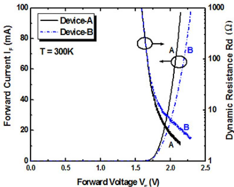
Figure 2 Forward I-V and dynamic resistance characteristics of the studied LEDs.
