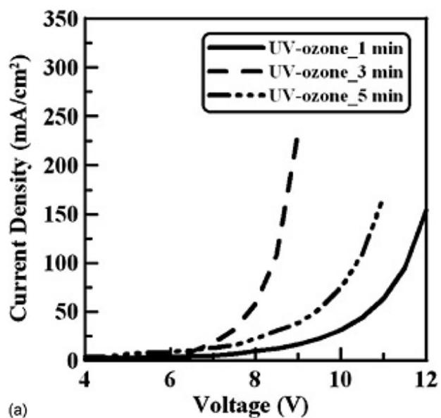
Fig. 2 The current density-voltage ( $J$ - $V$ ) characteristics of the studied TOLEDs under different UV-ozone exposure times for the Ag anode.
