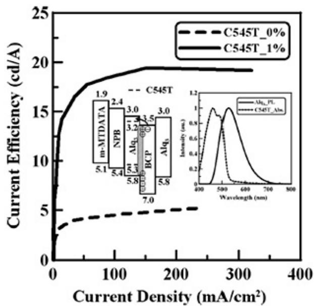
Fig. 3 Current efficiency-current density characteristics of the studied TOLEDs with/without the C545T doping. The insets are the energy-band diagram and the observed overlapping between the PL spectrum of Alq<sub>3</sub> and the absorption spectrum of C545T.
