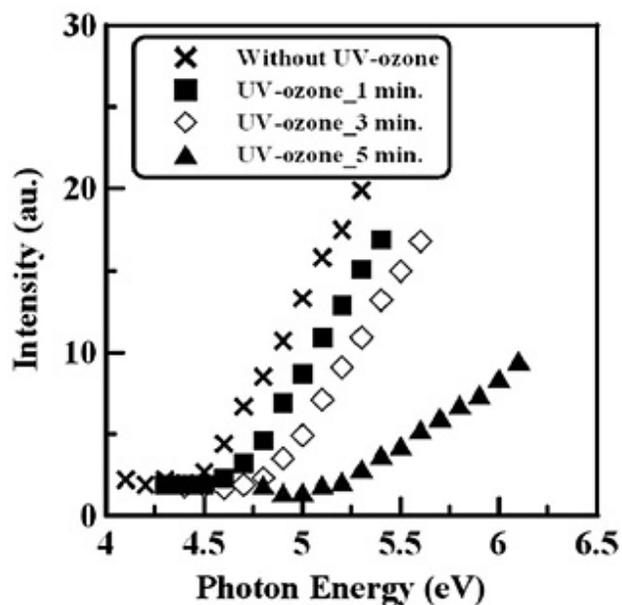
Fig.1 Photoelectron spectra of the UV-ozone-treated Ag anode under different exposure time
