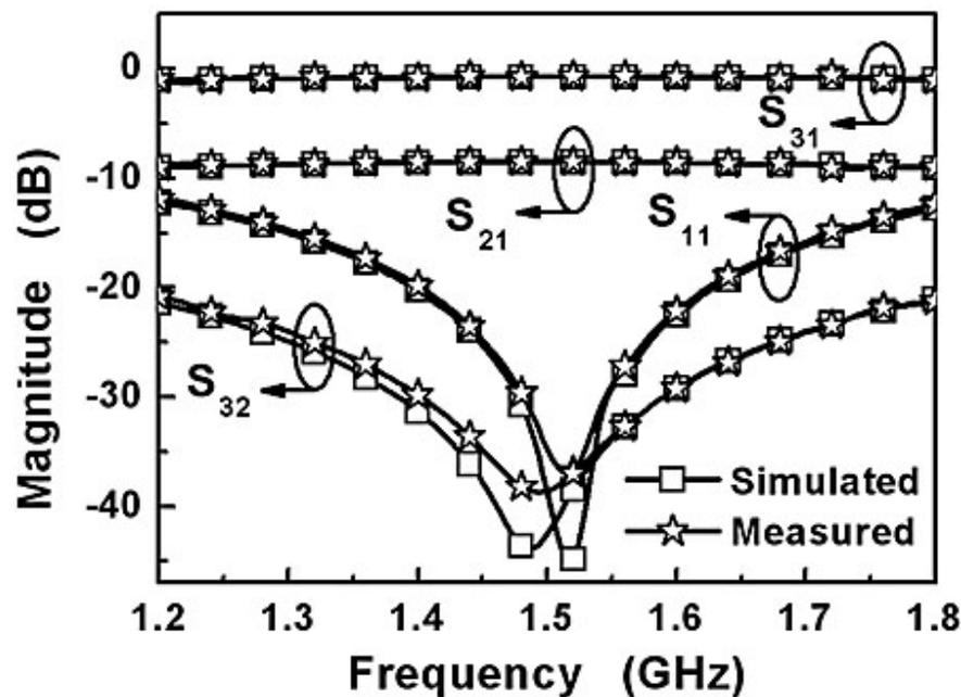
Figure 3. The simulated and measured results of the insertion loss, isolation, and input return loss as a function of frequency.
