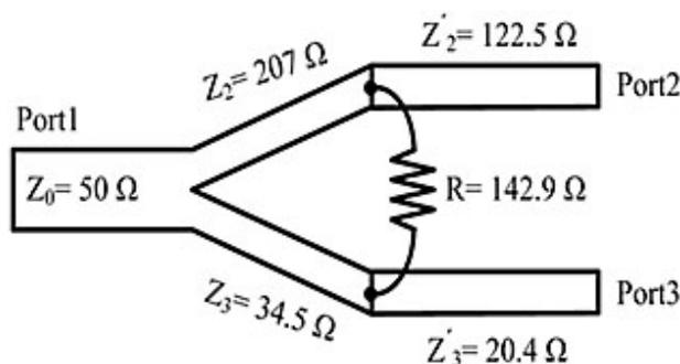
Figure 1. Topology of a 6:1 unequal Wilkinson power divider, including the required characteristic impedance, isolation resistor, and termination impedances.
