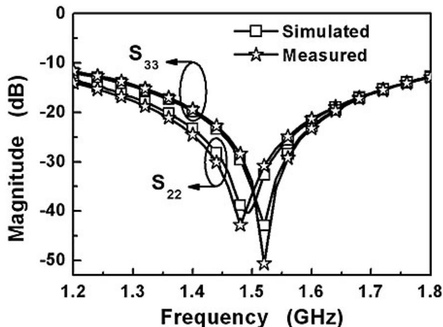
Figure 4. The simulated and measured results of the output return loss as a function of frequency.
