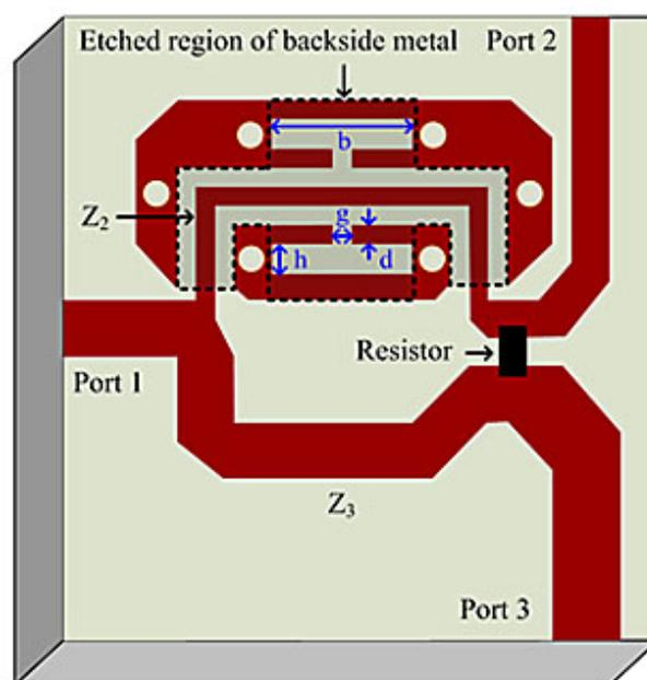
Figure 2. Schematic diagram of the proposed 6:1 unequal Wilkinson power divider.
