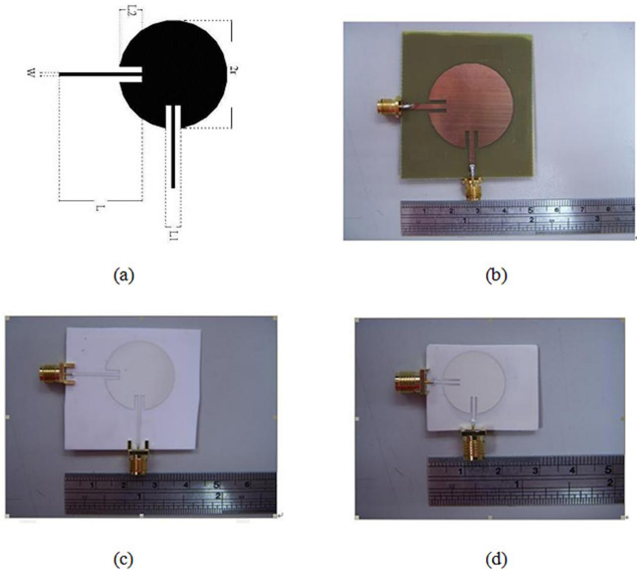
Fig. 1 The (a) physical layout of the designed circle dual-mode microstrip bandpass filter with a central frequency of 2.5 GHz, and fabricated ones on substrates using (b) FR4, (c) alumina, and (d) presented dielectric.
