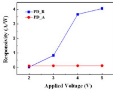
Fig. 3. Measured responsivity at 360 nm as a function of applied bias for both PDs.
