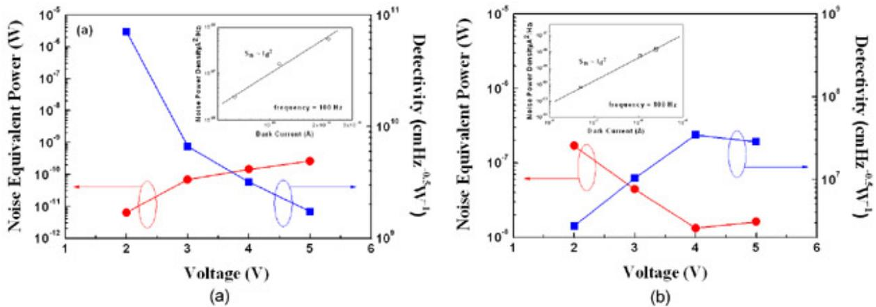
Fig. 5. Noise equivalent power ( $NEP$ ) and normalized detectivity ( $D^*$ ) of (a) PD\_A and (b) PD\_B. Insets show the corresponding noise power density measured at 100 Hz.
