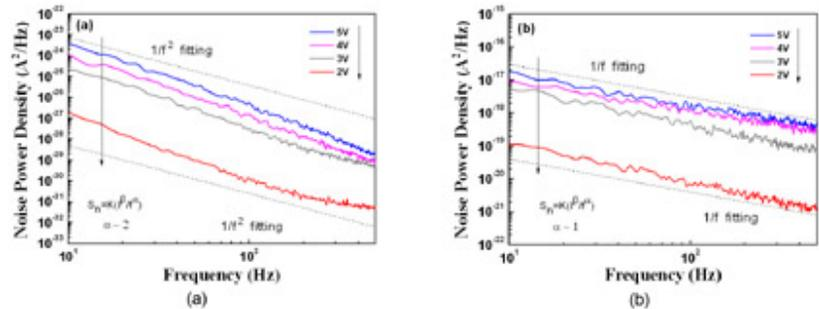
Fig. 4. Noise power spectra of (a) PD\_A and (b) PD\_B.
