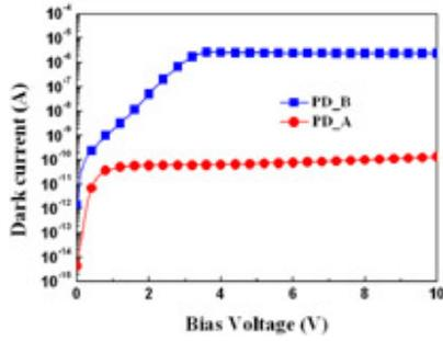
Fig. 1. Dark current-voltage characteristics of both fabricated MSM PDs.
