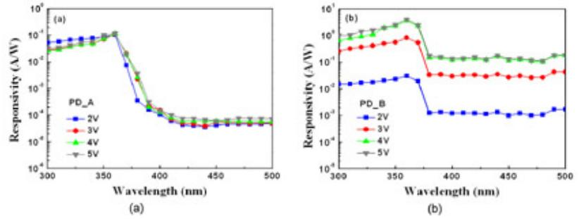
Fig. 2. Spectral responses at different bias of (a) PD\_A and (b) PD\_B.
