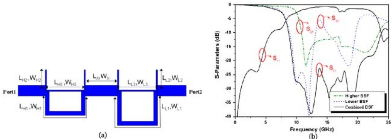
Figure 3. (a) Geometry and (b) simulated results of the combined BSF consists of higher BSF and lower BSF.
