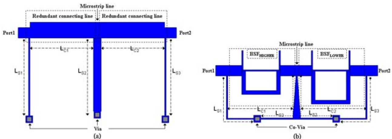
Figure 1. Geometry of (a) the traditional broadband BPF and (b) the proposed branch stubs co-via broadband bandpass filter with combined BSF substituted for redundant connecting lines.
