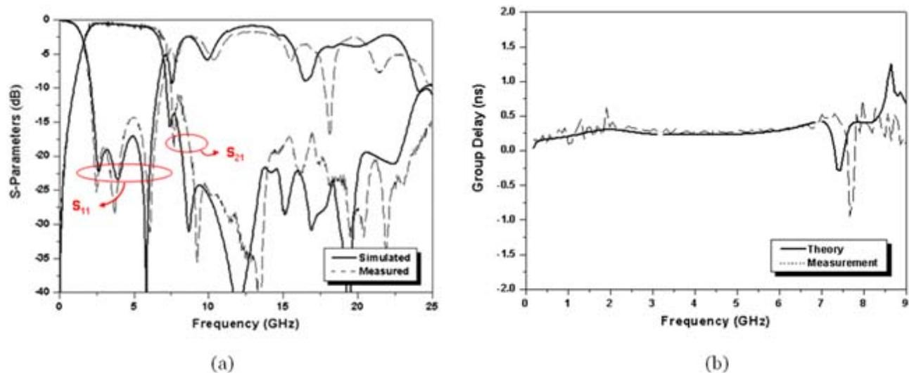
Figure 4. Measured and simulated (a) S-parameters and (b) Group delay of the proposed broadband BPF.
