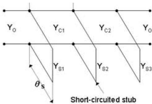
Figure 2. Circuit model for a pseudo distributed bandpass filter with three short-circuited stubs.
