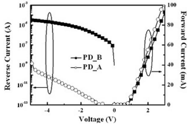
Figure 2 Room temperature I-V characteristics for the two fabricated PDs.
