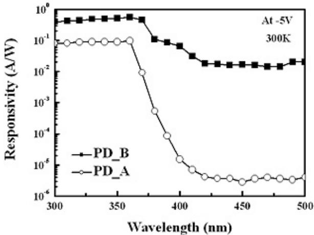
Figure 3 Room temperature spectral responsivity of both fabricated PDs biased at -5V.
