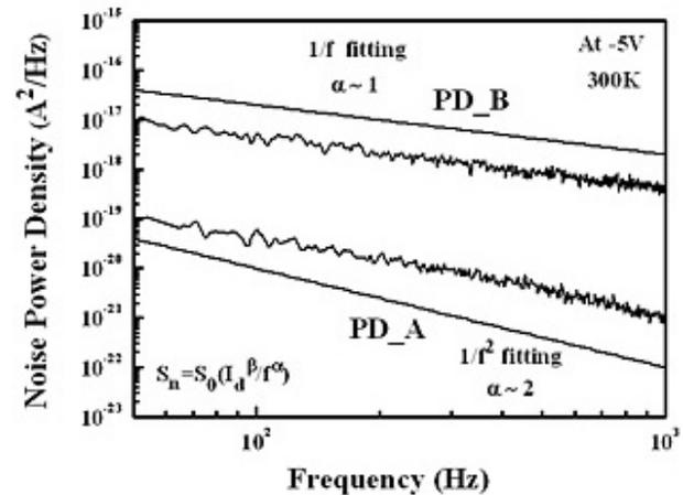
Figure 4 Measured noise power spectra of both fabricated PDs biased at -5V.
