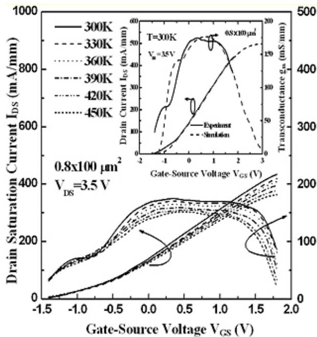
Fig. 3 Drain saturation current  $I_{DS}$  and extrinsic transconductance  $g_m$  versus gate-source voltage  $V_{GS}$  of the studied practical device at different temperatures. The inset shows experimental (solid lines) and simulated (dashed lines) results of drain saturation current  $I_{DS}$  and extrinsic transconductance  $g_m$  versus gate-source voltage  $V_{GS}$ .
