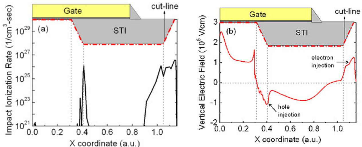
Fig. 3. Simulated (a) ii rate, (b) vertical electric field along the Si/SiO<sub>2</sub> interface under  $V_{ds} = 40$  V and  $V_{gs} = 12$  V.
