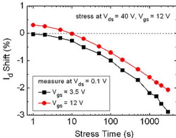
Fig. 4.  $I_d$  shift measured at different  $V_{gs}$  as a function of stress time for the device in Fig. 2.
