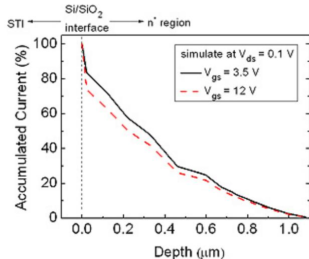
Fig. 5. Simulated accumulated current as a function of the depth from Si/SiO<sub>2</sub> interface at the location of bottom-left corner of STI.
