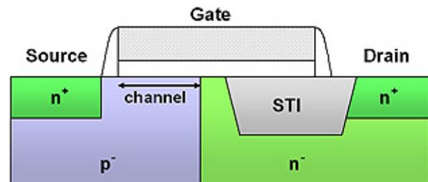
Fig. 1. Schematic cross section of the n-type LDMOS device used in this work.
