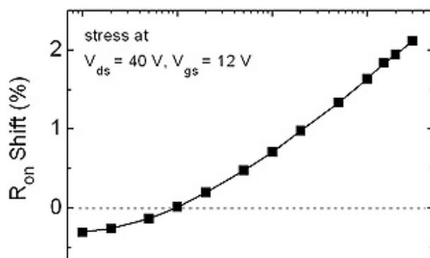
Two substrate current ( $I_{sub}$ ) peaks are observed in  $I_{sub}$ - $V_{gs}$  characteristics in our LDMOS devices. The first  $I_{sub}$  peak occurs at  $V_{gs} = 4$  V that is similar to the behavior in conventional MOSFETs. As  $V_{gs} > 8$  V,  $I_{sub}$  rises again because of Kirk effect and the second  $I_{sub}$  peak occurs at  $V_{gs} = 12$  V. When our LDMOS devices are stressed under
