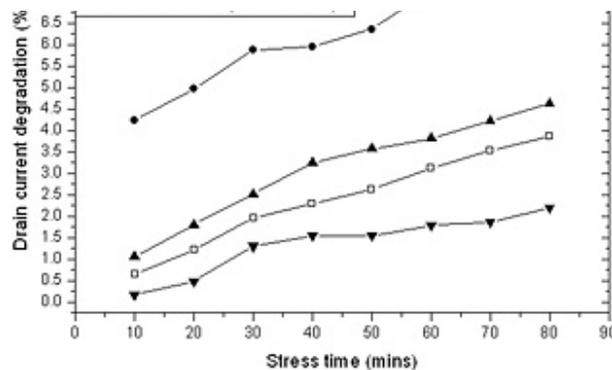
Fig. 2. Comparison of degradations of drain current in RF and DC stresses. (Measured at  $V_{gs}=1.2$  V and  $V_{ds}=1.8$  V)
