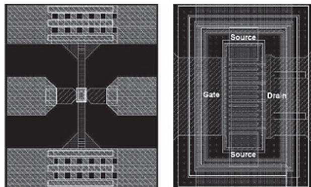
Fig. 1. (a) Layout pattern of the studied power cell. (b) Detail of the cell
