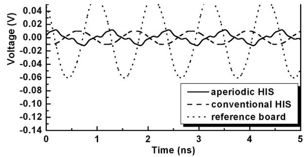
Figure 4. Time domain analysis for two high-impedance surface structures.
