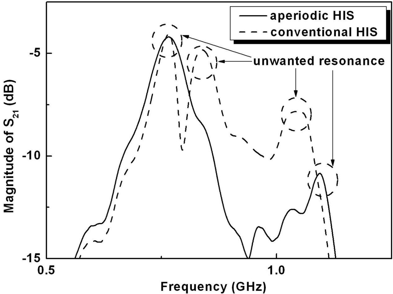
Figure 3. Compared with the suppression results in lower frequency range.
