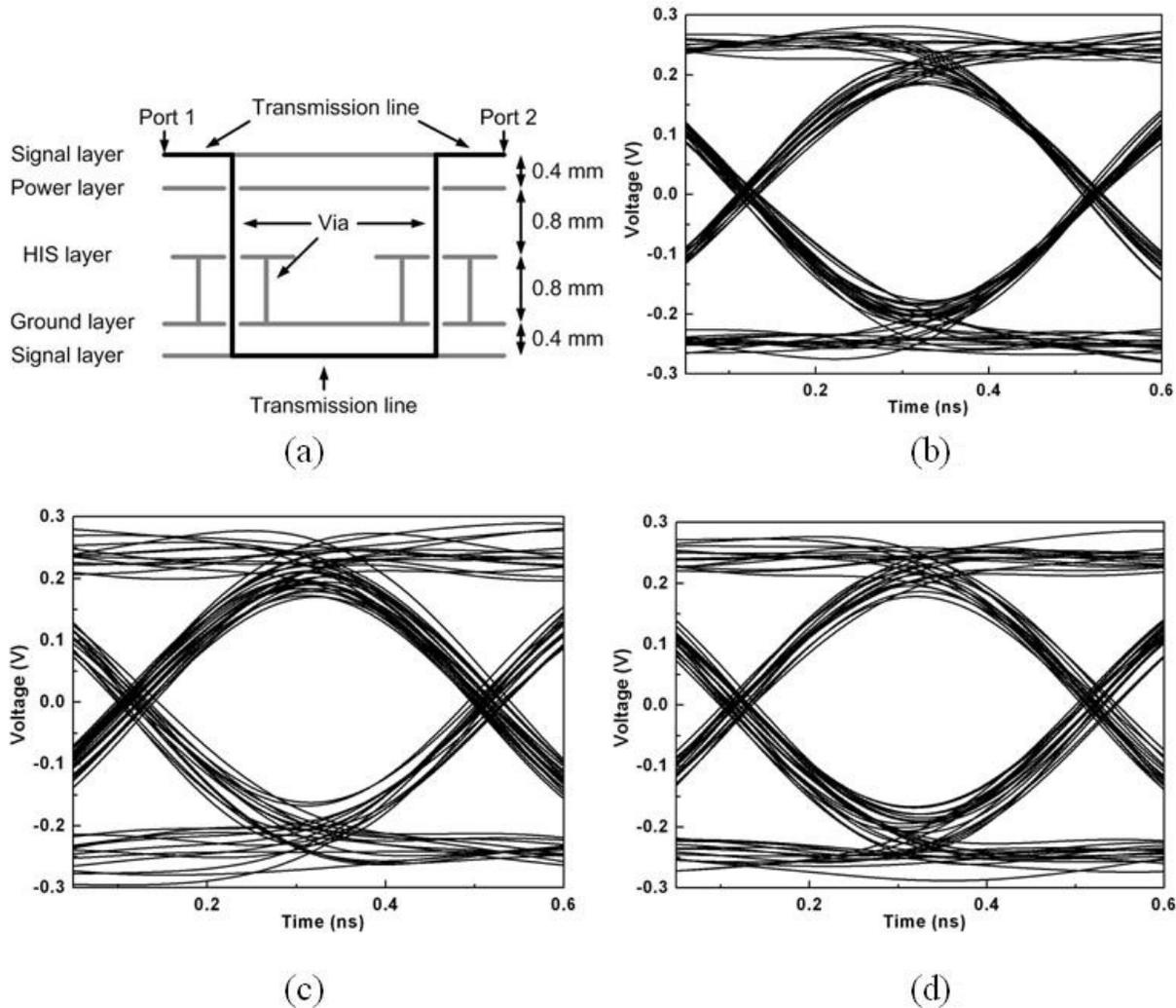
Figure 5. The eye diagram results. (a) Five layer structure for single-ended trace. (b) The reference board. (c) The conventional period structure. (d) The proposed aperiodic structure.
