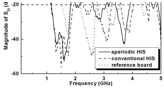
Figure 2. Compared with the suppression results between period and aperiodic high-impedance surface structure.
