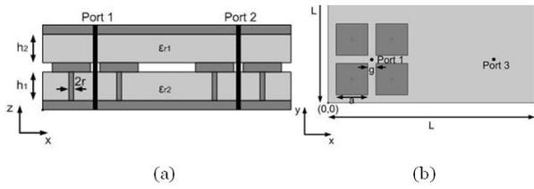
Figure 1. The schematic of the aperiodic high-impedance surface (a) side view, (b) top view.
