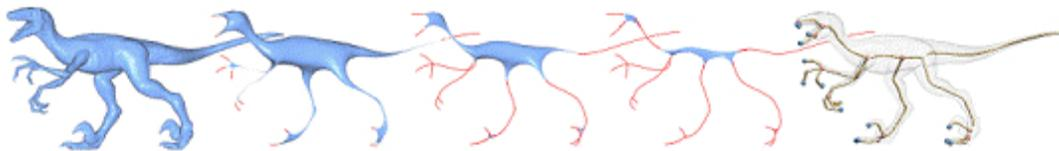
Figure 1. Left to right are the original raptor mesh and contraction results after 1, 2 and 3 iterations. The rightmost image shows the final skeleton after performing connectivity surgery and centeredness refinement [3].
