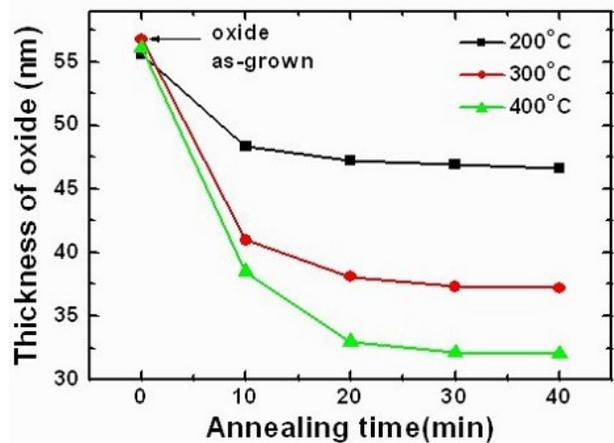
Fig. 3 Thicknesses of the oxide layers as a function of the thermal treatment time at various temperatures.
