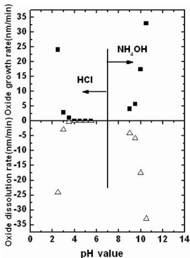
Fig. 1 The oxide growth rate and dissolution rate as a function of the pH value of the electrolytic solution. The PEC treatment time is 30 min.
