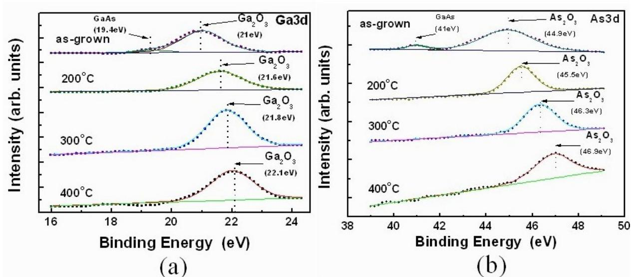
Fig. 4 XPS spectra for the core-level (a) Ga3d and (b) As3d of the PEC oxide layers, as-grown and annealed at various temperatures for 30 min.
