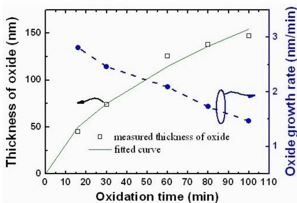
Fig. 2 The growth rate and thickness of the oxide layer produced on GaAs surface by PEC method at pH value of 3.5 as a function of oxidation time.
