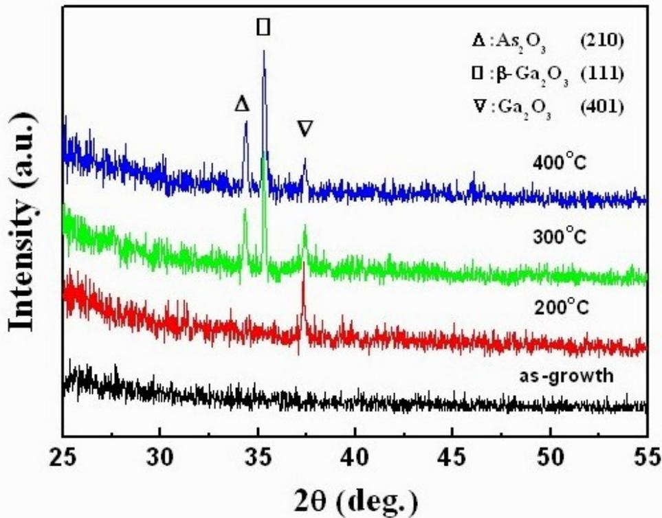
Fig. 5 X-ray diffraction patterns of the PEC oxide layers, as-grown and annealed at various temperatures for 30 min.
