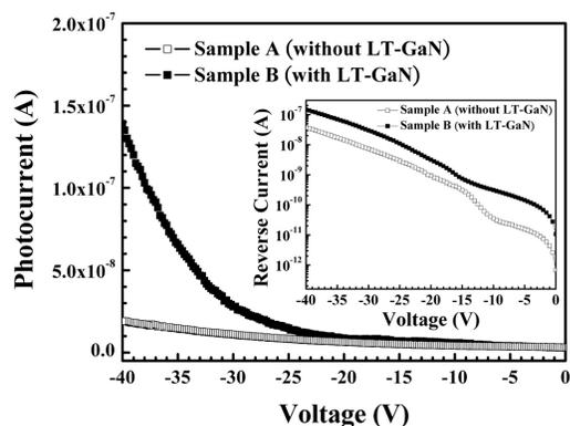
Figure 1. Measured photocurrent of photodiodes with (sample B) and without (sample A) LT-GaN interlayer under xenon light illumination. The inset
