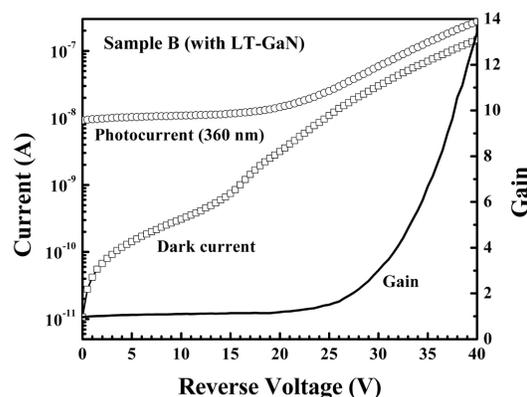
Figure 2. Reverse I-V characteristics of sample B in the dark and 360 nm light illumination. The right-
