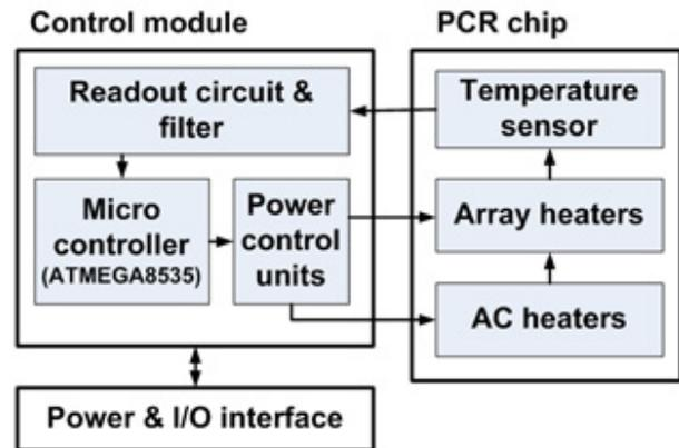
Figure 2 The block-diagram of AC-PCR system
