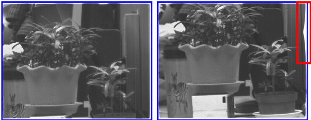
Fig. 3(a) The image taken in normal mode, (b) the image taken with a noisy transistor operating at 10 MHz.
