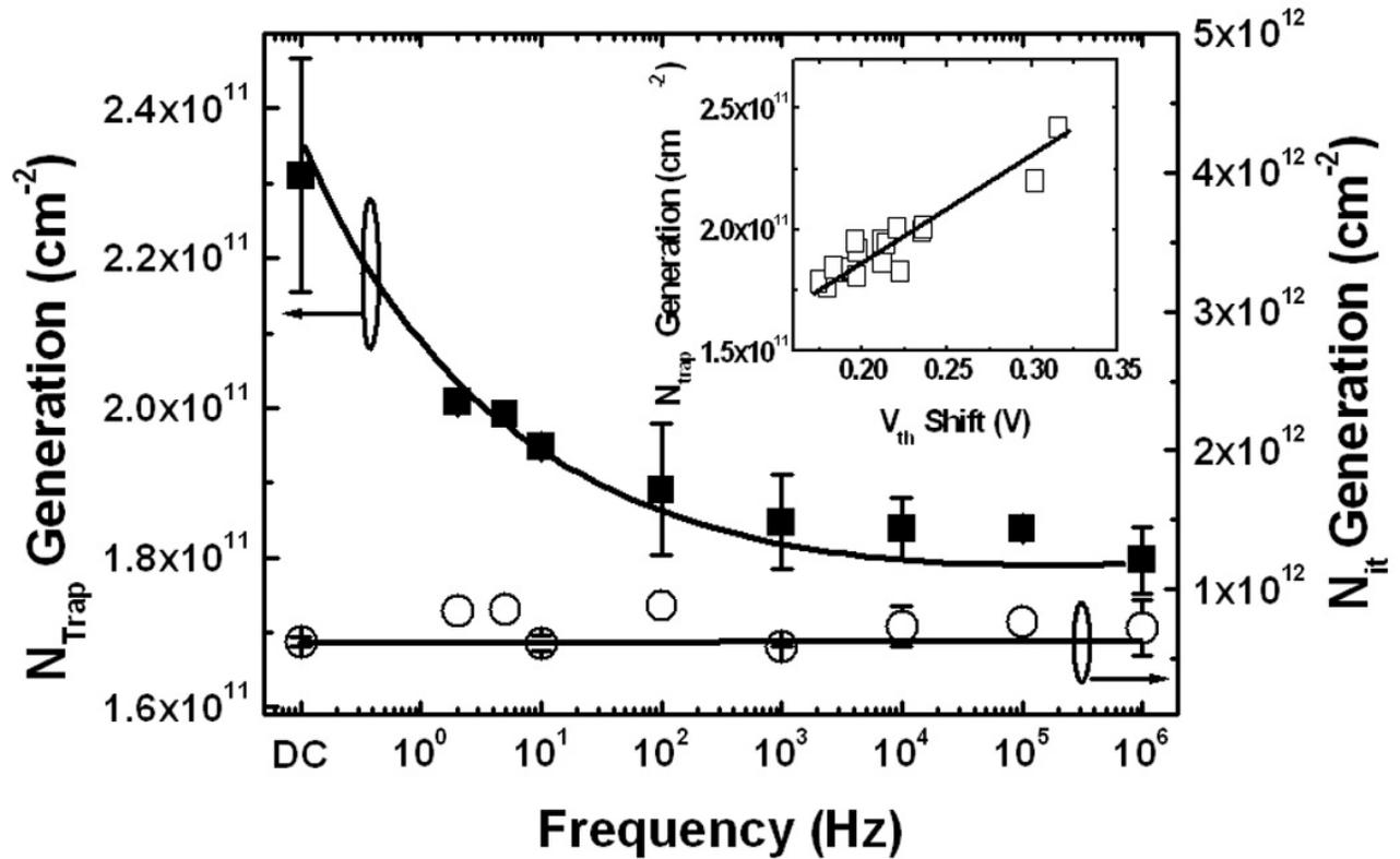
Fig. 2. The generation of  $N_{Trap}$  (square) and  $N_{it}$  (circle) under static and dynamic NBT stress as a function of stress frequency.
