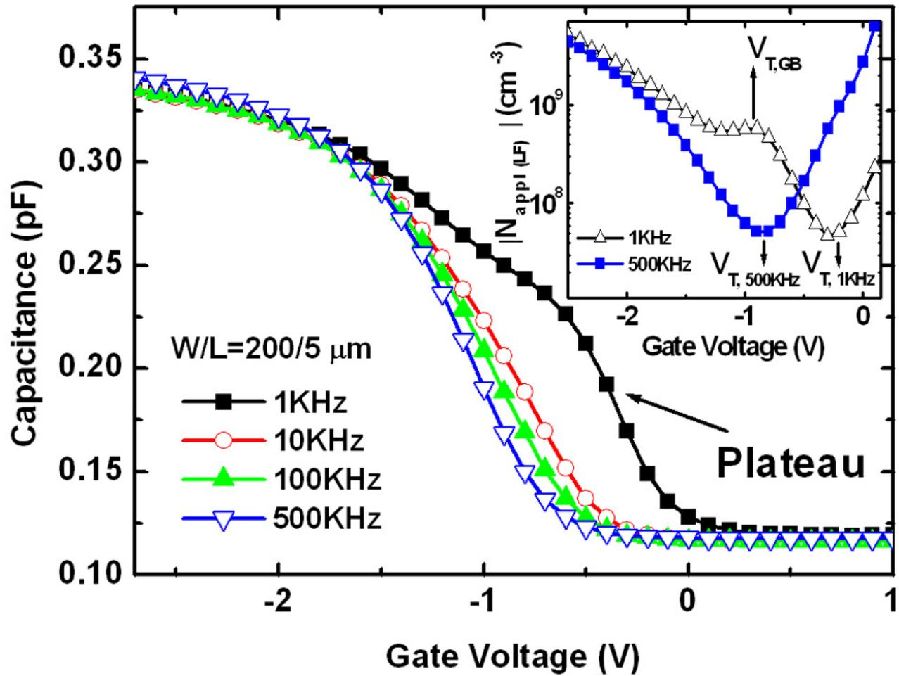
Fig. 3. The C-V characteristics of the LTPS TFTs. The inset shows the  $N_{\text{appl}}$  Vs gate bias.
