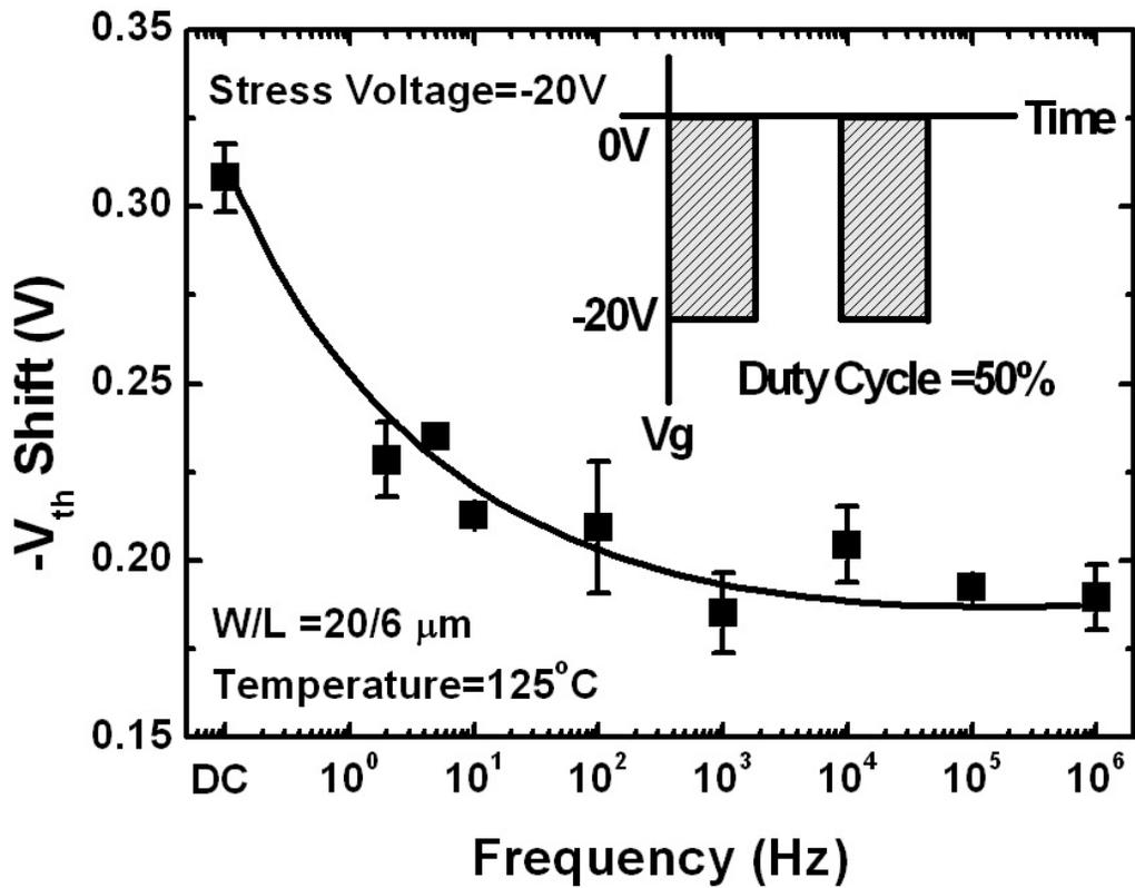
Fig.1. The negative threshold voltage shift ( $-\Delta V_{th}$ ) under static and dynamic negative bias temperature stress Vs stress frequency.
