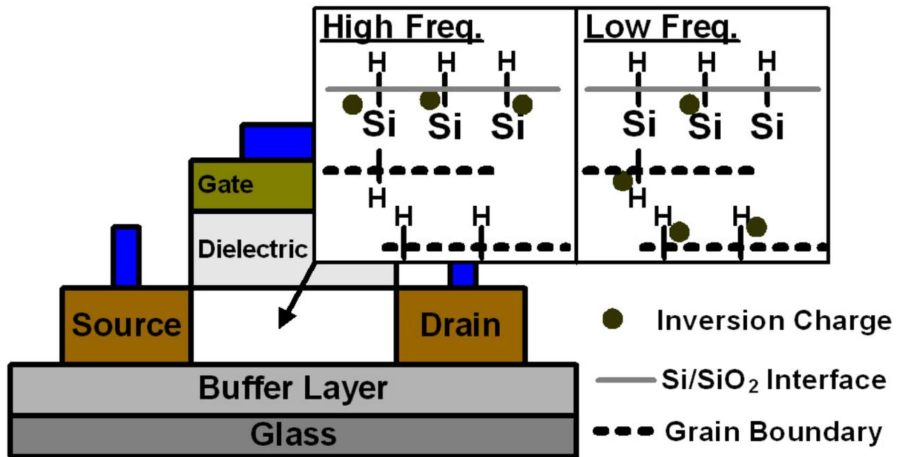
Fig. 4. Schematic diagram of LTPS TFT cross-section, and interaction between hydrogen atoms and inversion charges
