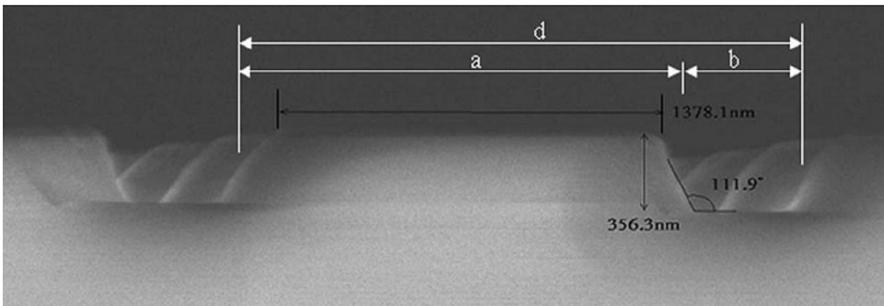
Fig2. SEM image of etching profile of the bottom pillar on the sapphire substrate.
