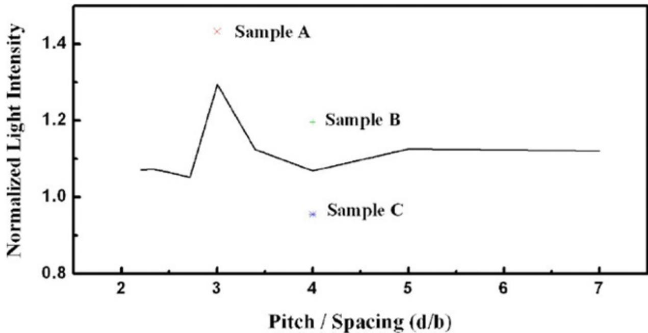
Fig3. The enhancement factor as a function of pitch to spacing ratio.
