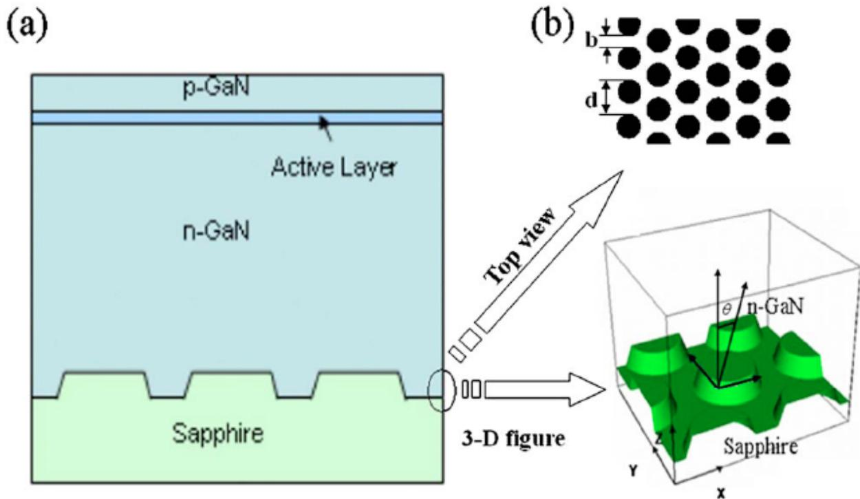
Fig1. Illustration for the GaN LED with bottom pillar structure
