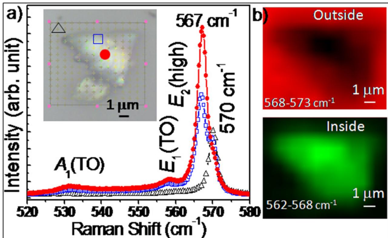
Fig. 2. a) Micro-Raman spectra for epi-GaN outside and different regions inside the indentation spot. Inset shows corresponding optical image of the indentation spot. b) Area mappings of outside and inside of the indentation spot, using different spectral regions indicated in the picture.
