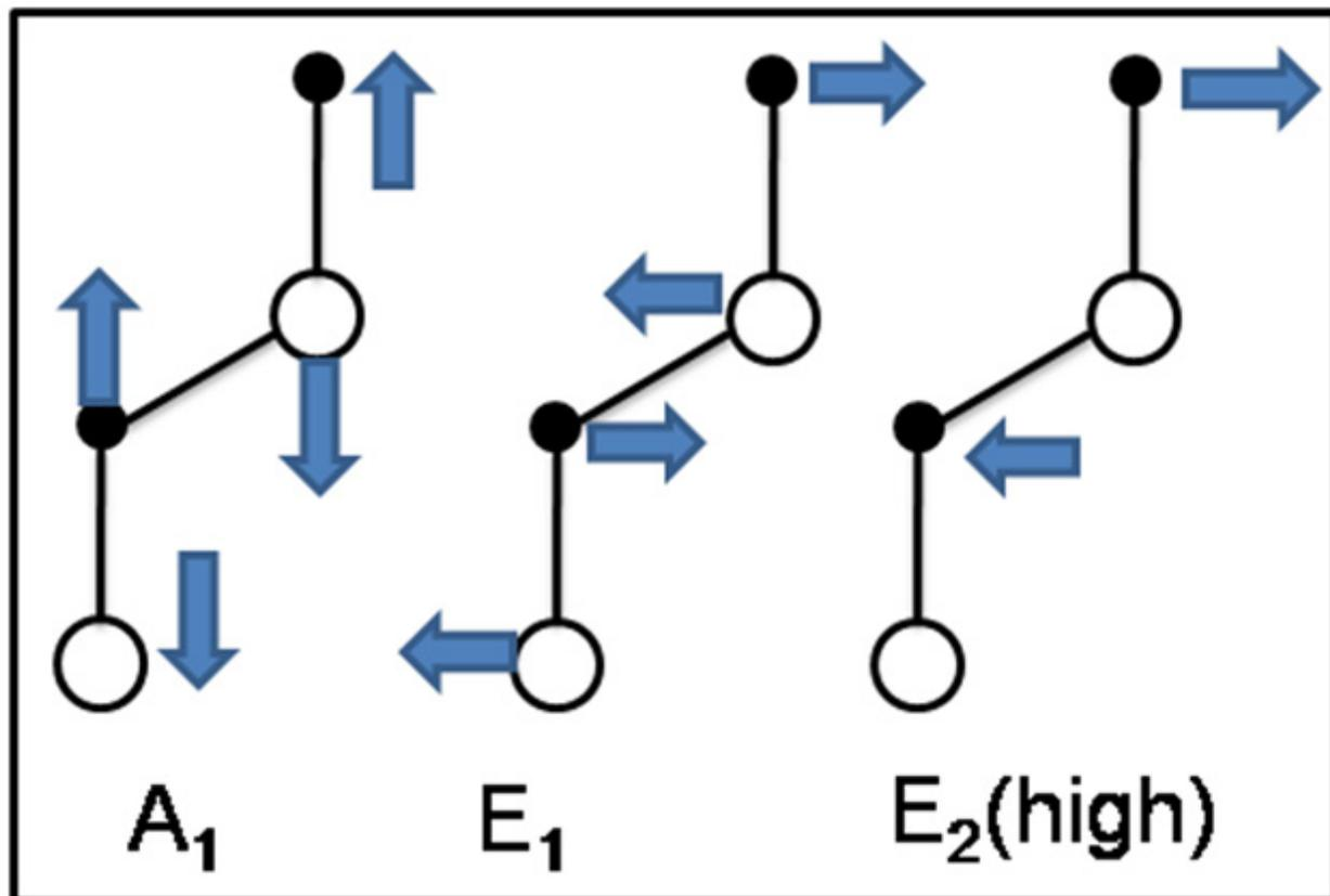
Fig. 4. Optical phonon modes in the wurtzite structure of GaN. Filled and unfilled symbols are represented by Ga and N, respectively. Arrows indicate directions of atomic vibrations.
