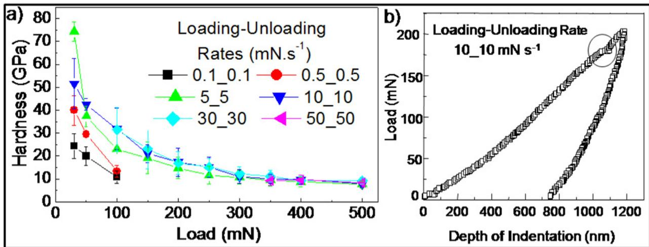
Fig. 1 a) Measured values of hardness of epi-GaN(0001) with load. Loading-unloading rate is also varied for the detailed studies. b) Typical loading-unloading lines at a fixed loading-unloading rate of 10 mN.s<sup>-1</sup>. The encircled regions are called as 'pop-in' burst.
