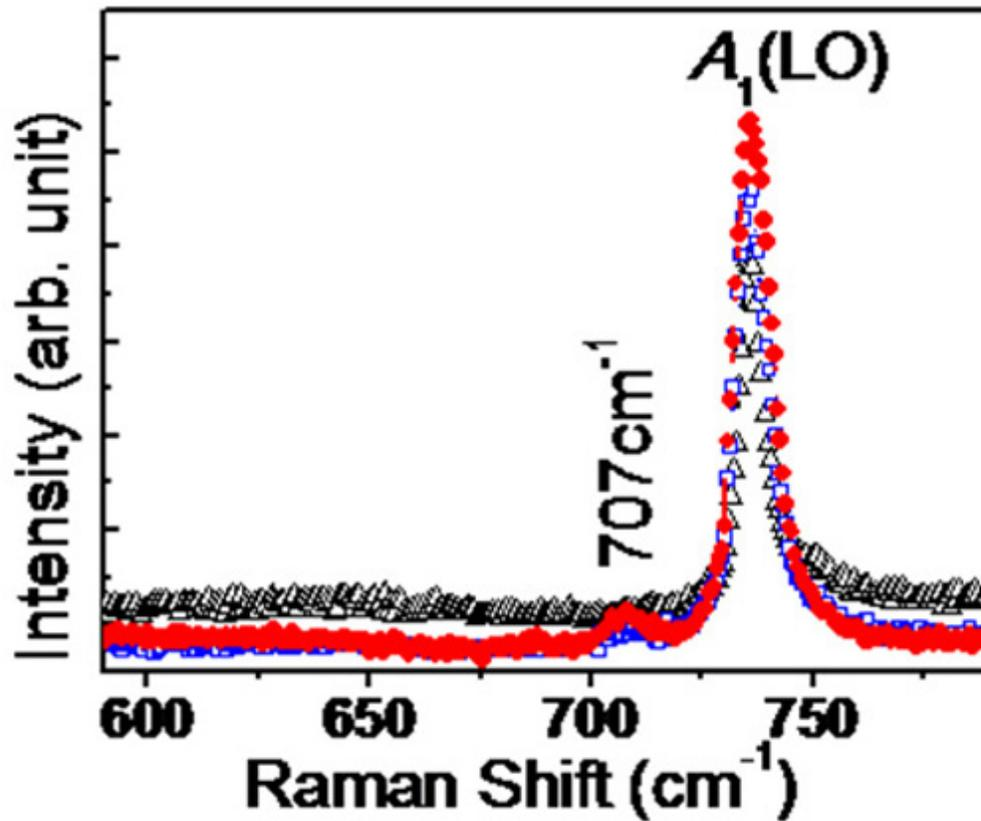
Fig. 3. Micro-Raman spectra for epi-GaN outside and different regions inside the indentation spot as shown in the inset of Fig. 2a.
