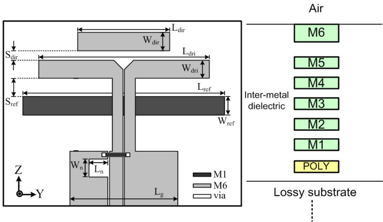
Fig.1 Schematics and cross-sectional view of the designed 60-GHz CPW-fed Yagi CMOS on-chip antenna.
