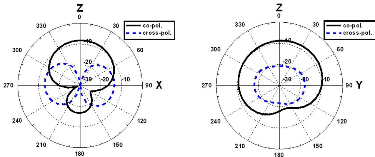
Fig.4 Simulated antenna radiation power patterns in the XZ-plane and YZ-plane at 60GHz.
