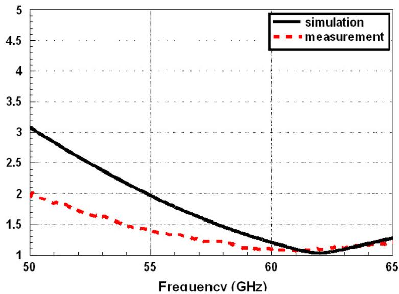
Fig.3 (a) CMOS antenna chip micrograph. (b) Simulated and measured antenna input SWR
