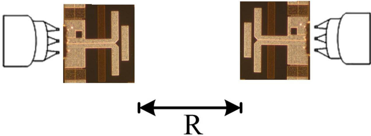
Fig.5 Illustration of the on-wafer measurement setup for the power gain of the on-chip antenna.
