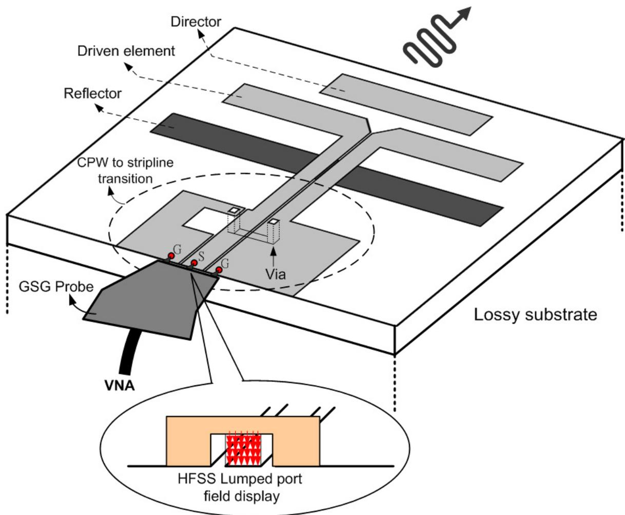
Fig.2 Illustration of HFSS port excitation of the on-chip antenna.
