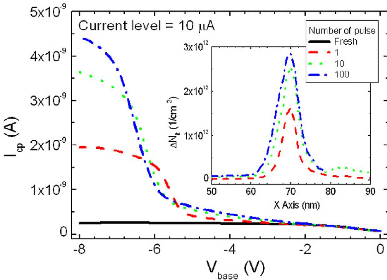
Fig. 3.  $I_{CP}$  data of the device before and after  $10\mu\text{A}$  current stressing for 100 pulses.  $\Delta N_{it}$  distribution is shown in the inset. The origin of X-axis in the inset is the poly-gate edge.
