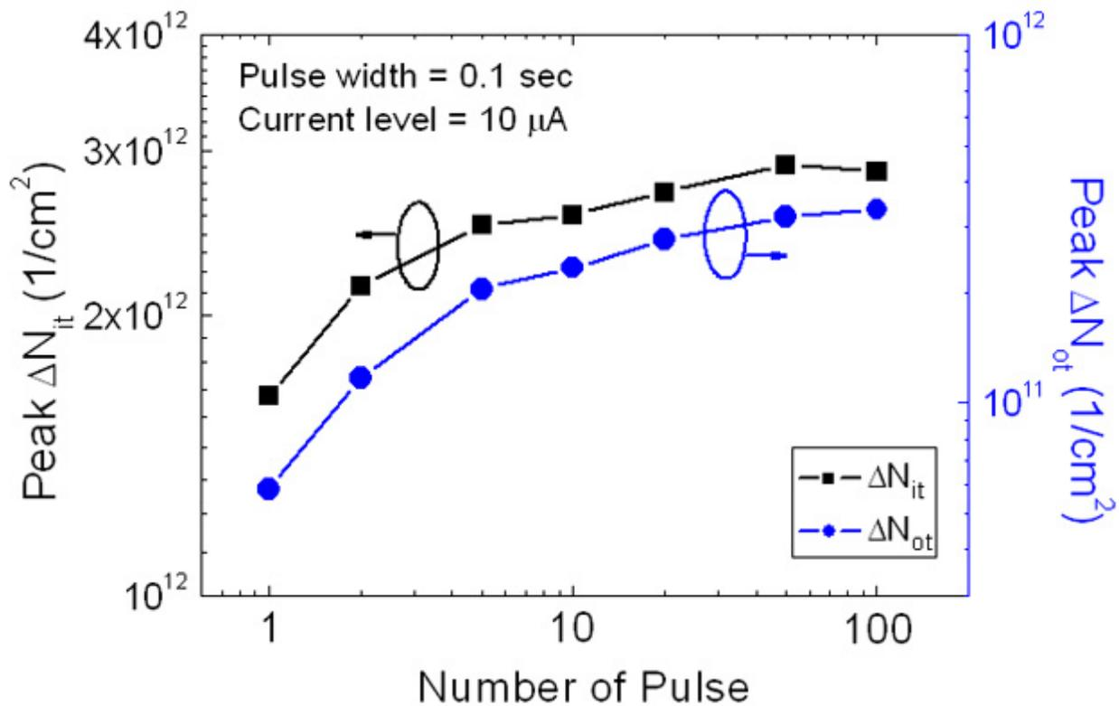
Fig. 4. The peak value of  $\Delta N_{it}$  and  $\Delta N_{ot}$  as a function of the number of current pulse.
