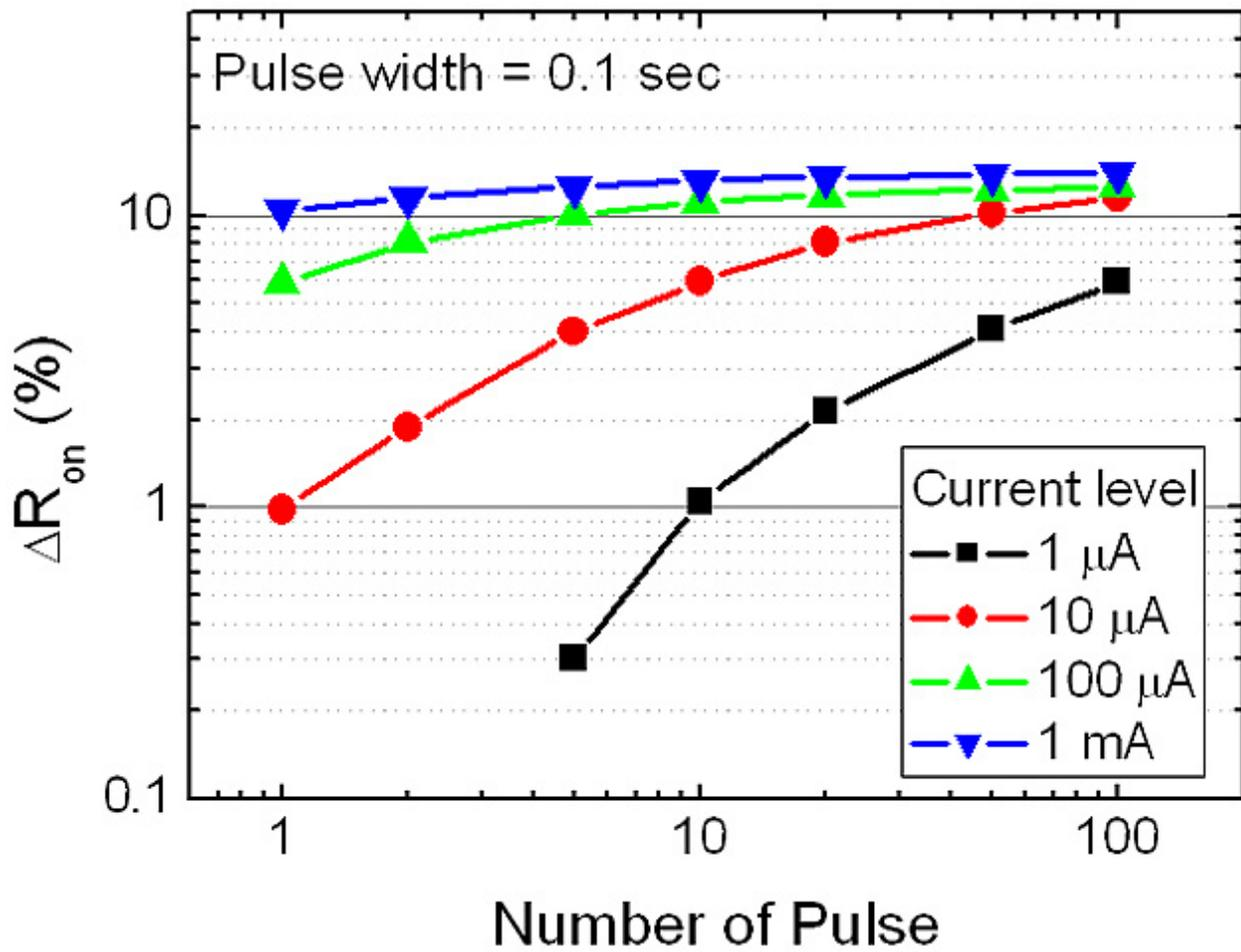
Fig. 2.  $R_{on}$  degradation as a function of the number of current pulse under various current levels.
