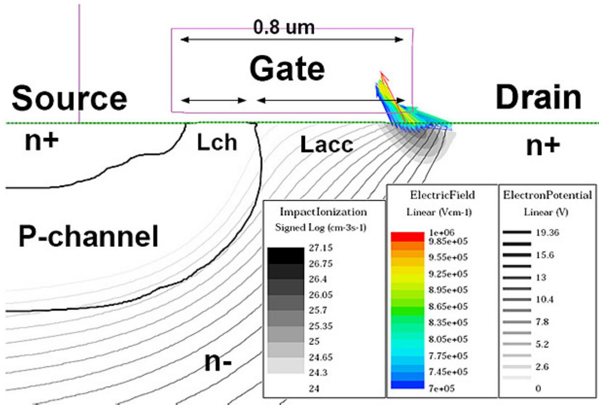
Fig. 1. The device cross section and TCAD simulation results on potential contour (line), impact ionization contour (field), and electric field (vector) of our LDMOS device under avalanche breakdown condition.
