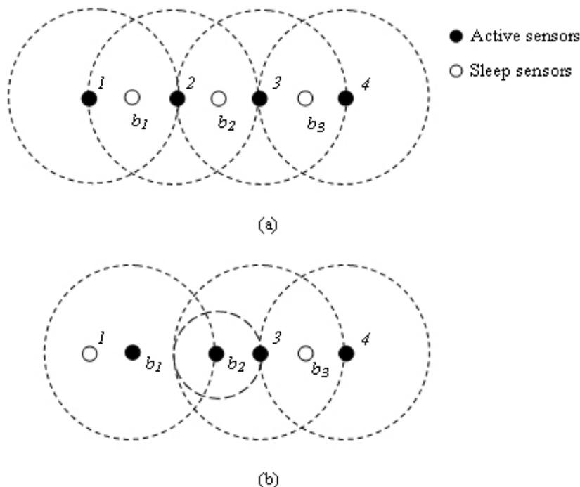
Figure 1: An example for  $P$ -CDS: (a) failure-free execution. (b) node 2 fails.
