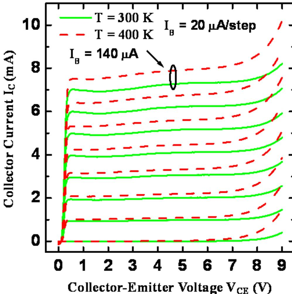
Fig. 3 Common-emitter current-voltage characteristics of the studied device at 300 and 400 K.
