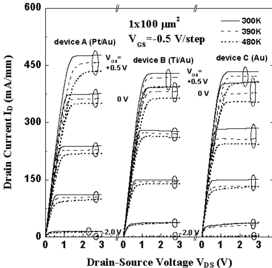
Fig. 2 Typical common-source I-V characteristics at different temperatures.
