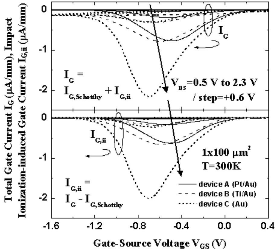
Fig. 3 The total gate current ( $I_G$ ) and impact ionization-induced gate current ( $I_{G,ii}$ ) versus gate-source voltage ( $V_{GS}$ ) under different drain-source voltage ( $V_{DS}$ ) at room temperature.
