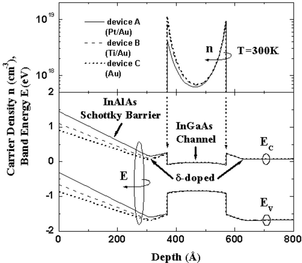
Fig. 1 Schematic band diagrams and calculated electron densities within channel layer regimes of the MHEMTs with different Schottky gate metals.
