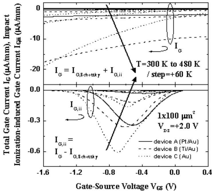
Fig. 4 The total gate current ( $I_G$ ) and impact ionization-induced gate current ( $I_{G,ii}$ ) versus gate-source voltage (VGS) at different temperatures.
