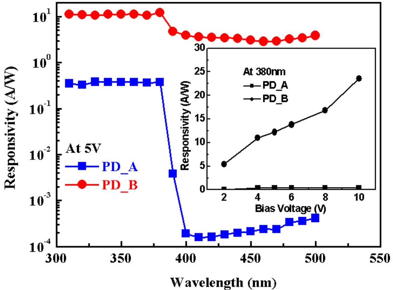
Fig. 4. Measured spectral responsivity of PD\_A and PD\_B measured at 5V bias voltage.
