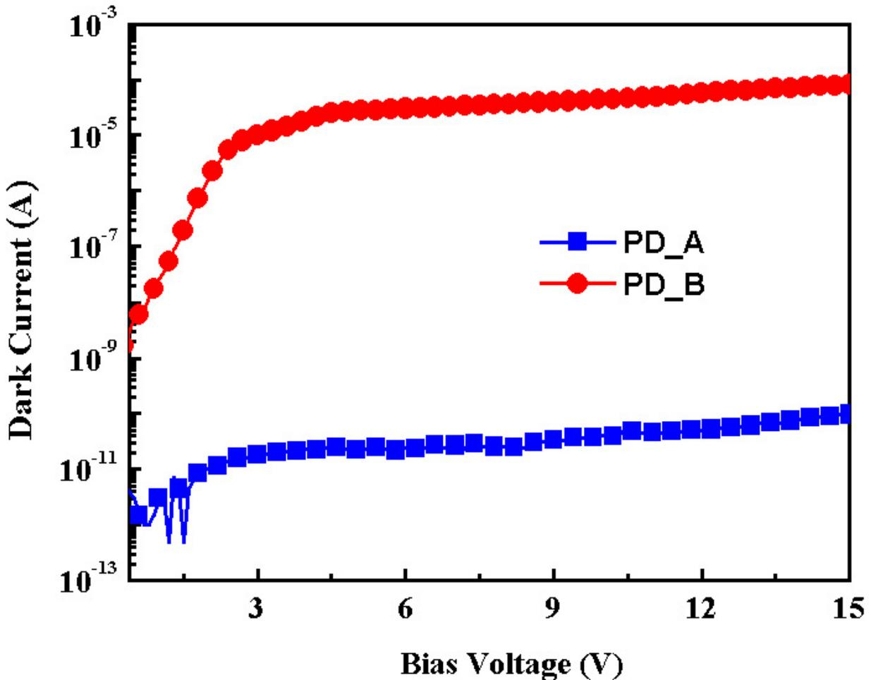
Fig. 3. The current-voltage characteristics of PD\_A and PD\_B under dark condition.
