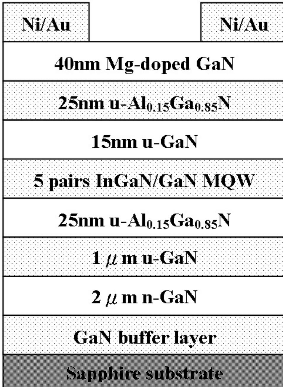
Fig. 1. The schematic diagram of the PD\_A.
