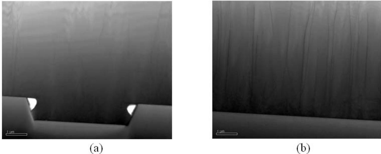
Fig. 1. Cross-sectional TEM micrographs of GaN epilayers grown on (a) PSS and (b) NSS, respectively.
