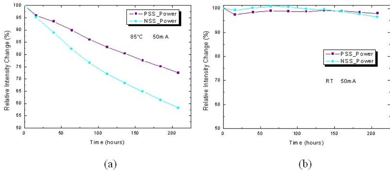
Fig. 2. Relative change in the intensity of PSS and NSS at (a) 85 ° C and also at (b) room temperature, for the final 208 hours.
