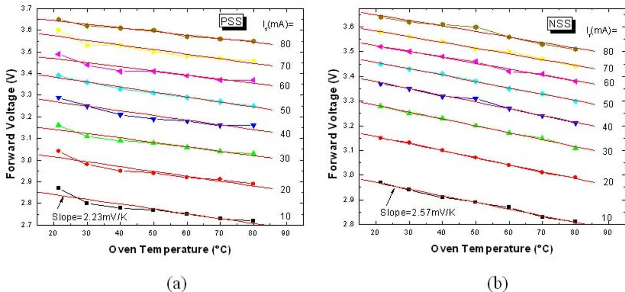
Fig. 3. Experimental forward voltage versus oven temperature for different pulse currents. A linear fit to the experimental data is also shown in (a) & (b).
