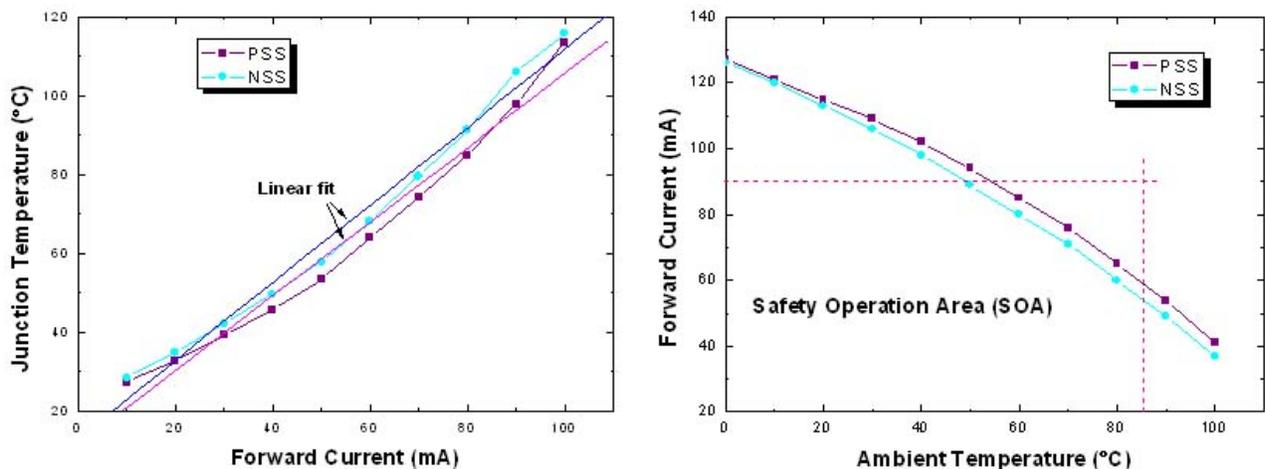
Fig. 4. (a) Junction temperature as a function of forward current for the PSS and NSS, and (b) the corresponding derating curves of the PSS and NSS LEDs.
