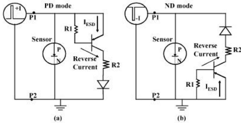
Fig. 2. Equivalent circuits of the module operated under (a) PD mode and (b) ND mode.
