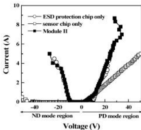
Fig. 3. ESD characteristics of Si-based ESD protection chip, AlGaN Schottky barrier sensor chip, and the entire module.
