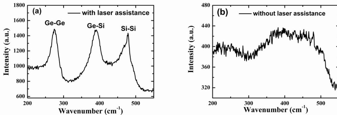
Fig.2 Raman spectra of SiGe films deposited (a) with and (b) without laser assistance
