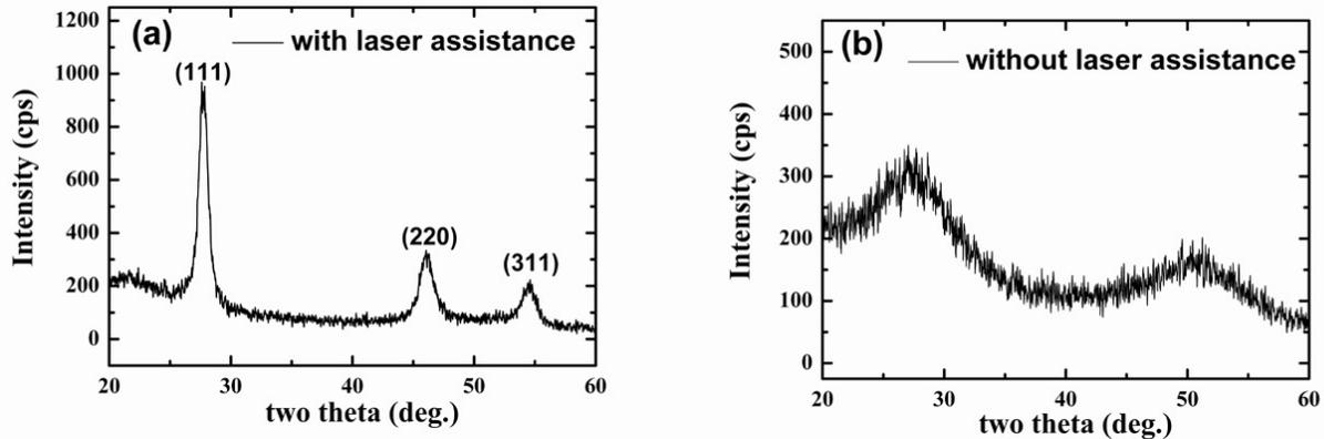
Fig.3 XRD diffraction patterns of SiGe films deposited (a) with and (b) without laser assistance
