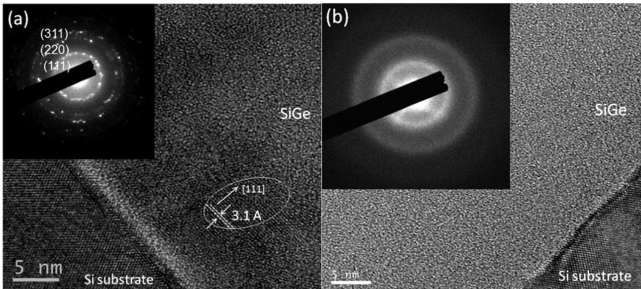
Fig.4 The selective area electron diffraction patterns of the HRTEM images of the SiGe films deposited (a) with and (b) without laser assistance
