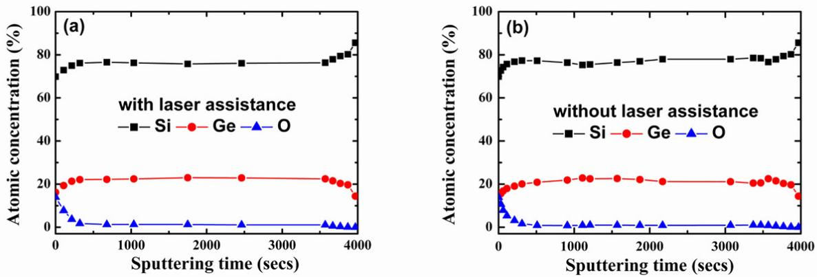
Fig.1 Auger electron spectroscopy depth profiles of SiGe films deposited (a) with and (b) without laser assistance
