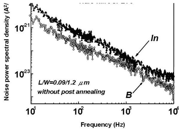
Fig. 5. Noise power spectral density ( $S_{Id}/I_d^2$ ) from 10 Hz to 10 kHz for 90 nm halo-implanted nMOSFETs with no post annealing.
