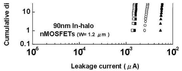
Fig. 7. Gate oxide leakage distributions for nMOSFETs with In- and B-halo structures under various post annealing treatments.
