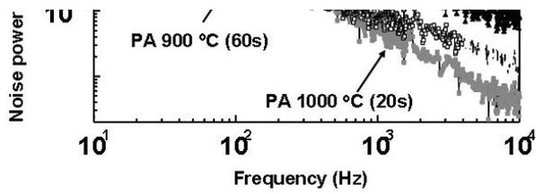
Fig. 6. Noise power spectral density ( $S_{Id}/I_d^2$ ) from 10 Hz to 10 kHz for 90 nm In-halo nMOSFET's under various post annealing treatments.
