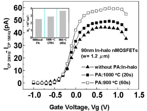
Fig. 8. Charge pumping currents for 90nm In-halo nMOSFETs under various post annealing treatments. The insert shows the  $N_{it}$  extracted from the  $I_{CP MAX}$ .
